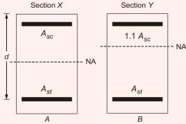
Due to presence of more compression steel in section Y, NA of section of Y is above than as of X. It means Y is more under-reinforced than X so ductility of Y is more. Since compression steel of Y is more so flexure resistance of X is less than as of Y.
