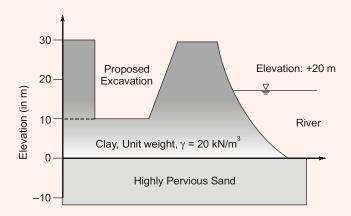
The water level in the adjacent river is at an elevation of +20.0 m. Unit weight of water is 10 kN/m<sup>3</sup>. The factor of safety (up to two decimal places) against sand boiling for the proposed excavation is \_\_\_\_\_
