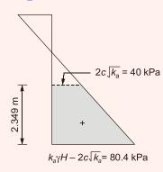
Earth pressure when tension cracks are developed
