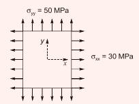
The Young's modulus of the material is  $2 \times 10^{11}$  N/m<sup>2</sup> and the Poisson's ratio is 0.3. If  $\sigma_{_{77}}$  is negligibly small and assumed to be zero, then the strain  $\epsilon_{_{77}}$  is
