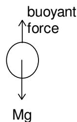
Resultant force =  $B - Mg = Mg/2$  (upward)
