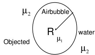
Substituting value in equation (1) and (2) the final image is formed at  $\frac{2R}{3}$  and it is virtual image
