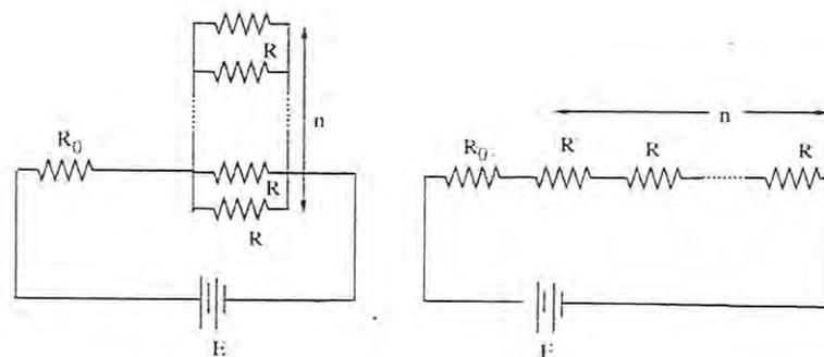
The batteries in both circuits are identical and net power dissipated in the  $n$  resistors in both circuits is same. The ratio  $R_0/R$  is
