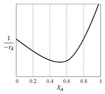
Which amongst the following reactor configurations gives the lowest total volume of the reactor(s)?
