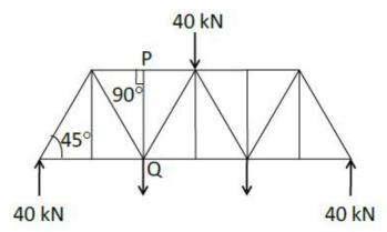
For a symmetrical two dimensional truss as shown in the above figure, vertical force in kN acting on the member PQ is \_\_\_\_\_
