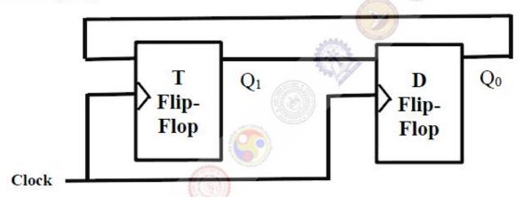
Initially, both Qo and Q1 are set to 1 (before the 1st clock cycle). The outputs
