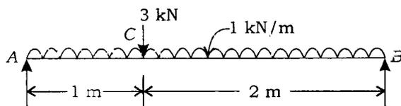
If ISJB 150 with  $I_{XX} = 300 \text{ cm}^4$  is used for the beam, the maximum value of bending stress is
