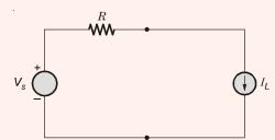
The value of  $I_L$  that maximizes the power absorbed by the constant current load is
