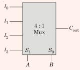
Which one of the following statements correctly describes the choice of signals to be connected to the inputs  $I_0$ ,  $I_1$ ,  $I_2$  and  $I_3$  so that the output is  $C_{out}$ ?
