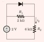
The magnitude of the current  $i_2$  (in mA) is equal to\_\_\_\_\_
