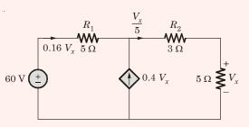
Using KVL in the outer loop
