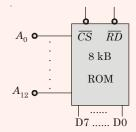
: 13 Address lines are required for memory chip. But the address range given as 1000 H - 2FFF H
