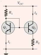
The value of  $R_2$  (in  $\Omega$ ) for which  $I_2 = 100 \ \mu A$  is \_\_\_\_\_
