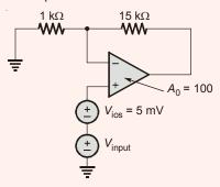
The output voltage (in millivolts) is \_\_\_\_\_
