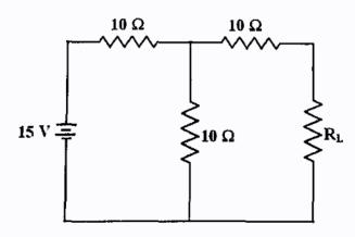
Assuming an ideal voltage source, Thevenin's resistance and Thevenin's voltage respectively for the above circuit are
