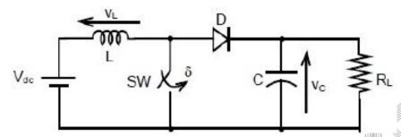
Under steady state operating conditions, the average voltage across the inductor and the capacitor respectively, are
