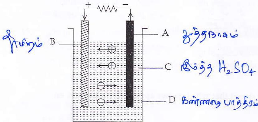
Volta cell diagram is given below. Label the parts A, B, C and D.
