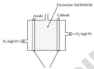
Porous carbon or graphite electrodes impregnated with black Pt particles
