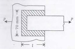
The maximum tensile and shear stresses are 70 N/mm<sup>2</sup> and 56 N/mm<sup>2</sup> respectively. The plate is 70 mm wide and 12.5 mm thick. What will be the value of l if the total load carried by the joint is 85 kN?
