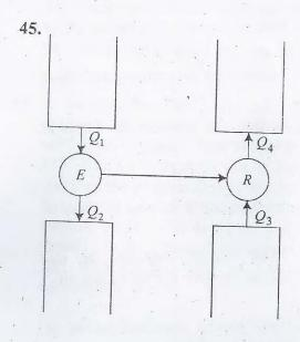
In the figure shown above, E is the heat engine with efficiency of 0.4 and R is the refrigerator. If  $Q_2 + Q_4 = 3Q_1$ , the COP of the refrigerator will be
