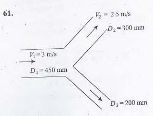
In the above layout of piping, what is the velocity in 200 mm diameter pipe?
