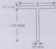
For the depth of plastic neutral axis from the top of the T-section to be 9-583 mm, the flange width b must
