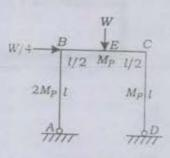
What is the bending moment at Bat collapse conditions?
