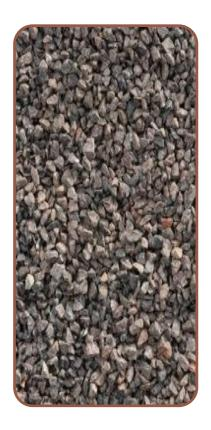
Aggregate is the component of a composite material that resists compressive stress and provides bulk to the composite material. Typically include both sand and gravel.
