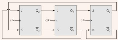
The above synchronous sequential circuit built using JK flip flops initialized with  $Q_{9}Q_{1}Q_{0} = 000$ . The state sequence for this circuit for the next three clock cycles is
