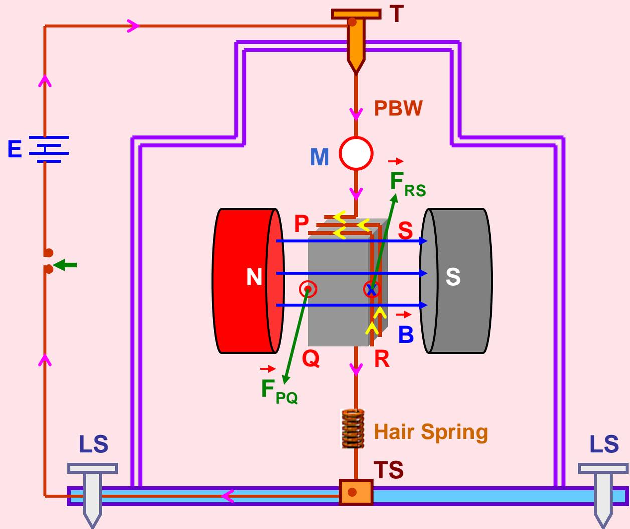
T – Torsion Head, TS – Terminal screw, M – Mirror, N,S – Poles pieces of a magnet, LS – Levelling Screws, PQRS – Rectangular coil, PBW – Phosphor Bronze Wire
