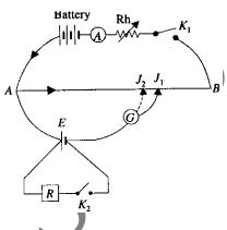
Since the values of  $l_1$ ,  $l_2$ , and R are known, the value of the internal resistance r of the cell can be determined.
