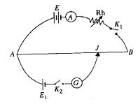
and can make contact at any point on the wire. The potentiometer is said to be balanced if there is no current in the galvanometer. The potential gradient across the wire (k = V/I) is constant. Sensitivity of a potentiometer can be increased by decreasing potential gradient i.e. by increasing length of wire.
