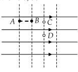
The distance between A and B is same as that between C and D. But, A and B will have some potential difference, whereas C and D being on the same equipotential, will have no potential difference. Hence, (b) is not correct.
