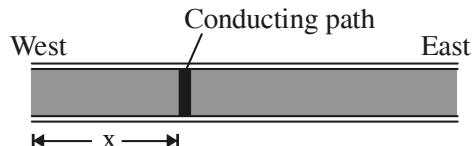
The resistance of the wires and the short is then  $100\Omega$  when the measurement is made from the east end,  $200\Omega$  when it is made from the west end. What is value of  $R$  (in deca ohm).
