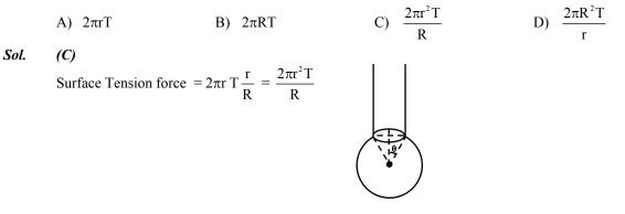
51. If  $r = 5 \times 10^{-4}$  m,  $\rho = 10^3$  kg m<sup>-3</sup>, g = 10 m/s<sup>2</sup>, T = 0.11 Nm<sup>-1</sup>, the radius of the drop when it detaches from the dropper is approximately
