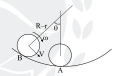
$$E = mg(R-r)(1-\cos\theta) + \frac{1}{2} \times \frac{1}{2}mr^{2} \times \left(\frac{R-r}{r}\right)^{2} \left(\frac{d\theta}{dt}\right)^{2} + \frac{1}{2}m \times (R-r)^{2} \left(\frac{d\theta}{dt}\right)^{2}$$
