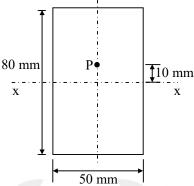
The maximum bending stress produced in the bar at xx is nearly
