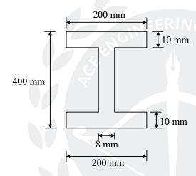
If the permissible stress is  $150 \text{ N/mm}^2$ , the bending moment M will be nearly
