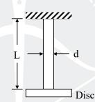
The system can be simplified as simple spring mass system (neglecting mass of shaft)
