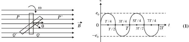
As coil rotates, the magnetic flux through the coil changes with time. Hence e.m.f induced in the coil is given by
