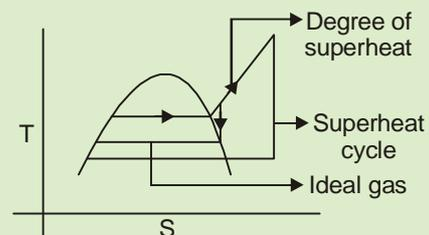
By increasing maximum pressure moisture content of turbine exhaust will be less, compare to ideal cycle.
