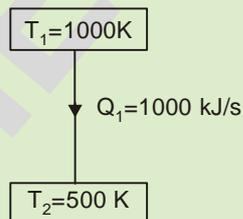
According to guoy stodola's theorem, loss of available energy
