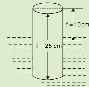
Buoyancy force = weight of water displaced
