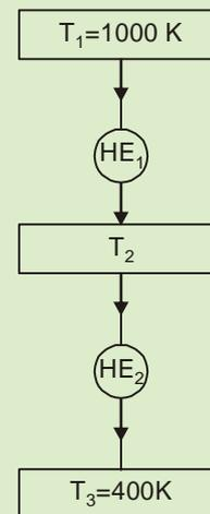
$$\left( 1 - \frac{T_2}{1000} \right) = \left( 1 - \frac{400}{T_2} \right)$$
