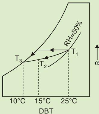
$$\begin{aligned} \text{BPF} &= \frac{T_1 - T_2}{T_1 - T_3} \\ &= \frac{25 - 15}{25 - 10} = \frac{10}{15} = \frac{2}{3} \\ &= 0.67 \end{aligned}$$
