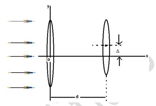
Taking the origin of coordinates, O, at the centre of the first lens, the x and y-coordinates of the focal point of this lens system, for a parallel beam of rays coming from the left, are given by
