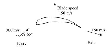
The magnitude of absolute velocity at entry is 300 m/s at an angle of 65° to the axial direction, while the magnitude of the absolute velocity at exit is 150 m/s. The exit velocity vector has a component in the downward direction. Given that the axial (horizontal) velocity is the same at entry and exit, the specific work (in kJ/kg) is
