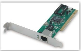
**Network interface cards**, commonly referred to as NICs, and are used to connect a PC to
