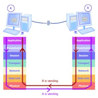
It provides a description of how network hardware and software work together in a layered fashion to make communications possible. It also helps with trouble shooting by providing a frame of reference that describes how components are supposed to function.
