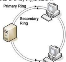
**FDDI (Fiber-Distributed Data Interface)** is a standard for data transmission on fiber optic lines in a local area network that can extend in range up to 200 km (124 miles). The FDDI protocol is based on the token ring protocol. In addition to being large geographically, an FDDI local area network can support thousands of users.
