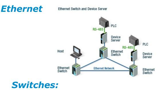
**Ethernet switches** are an expansion of the concept in Ethernet bridging. LAN switches can link four, six, ten or more networks together, and have two basic architectures: cut-through and store-and-forward. In the past, cut-through switches were faster because they examined the packet destination address only before forwarding it on to its destination segment. A store-and-forward switch, on the other hand, accepts and analyzes the entire packet before forwarding it to its destination.
