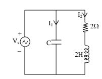
In the network shown above  $V_s = 4$ cos 2t. The value of C is so chosen the circuit impedance is that maximum. Then  $I_1$  leads  $I_2$  by (a) 45° (b) 90° (c)  $0^{\circ}$ (d) 135°
