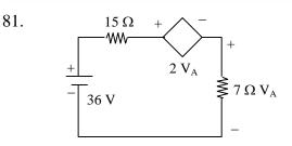
The power dissipated in the controlled source of the network shown above is
