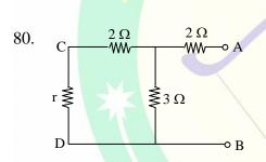
For the circuit shown above the above the value of r connected between C and D is such that the equivalent resistance of the circuit by looking into circuit through terminals A and B is r only. Then the value of r is
